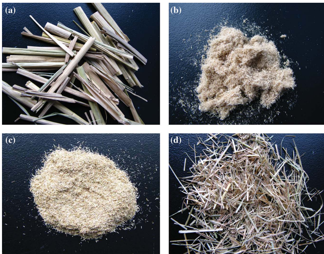
Figure 1 The morphology of rice straw (a) rice straw, (b) rice straw refined fiber, (c) rice straw ground pellets, and (d) rice straw strand. [Color figure can be viewed in the online issue, which is available at wileyonlinelibrary.com .]
